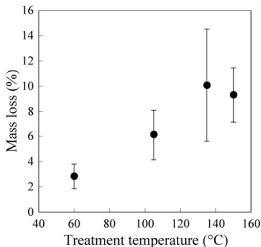
Fig. 4 Effect of treatment temperature on durability against the termite, *C. formosanus*. Samples were heated for 72 hours. Percentage of mass loss was calculated from the sample exposed to *C. formosanus* for 8 weeks. Bars indicate standard deviation (n=6).
