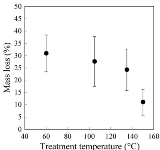
Fig. 2 Effect of treatment temperature on durability against the brown-rot fungus, *Fomitopsis palustris*. Heat-treatment were carried out for 24 hours. Percentage of mass loss was calculated from the sample exposed to the fungus for 8 weeks. Bars indicate standard deviation ( $n=12$ ).
