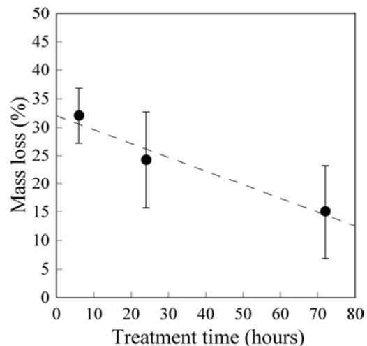
Fig. 3 Effect of treatment time on durability against the brown-rot fungus, *Fomitopsis palustris*. Heat-treatment were carried out at 135 °C. Percentage of mass loss was calculated from the sample exposed to the fungus for 8 weeks. Bars and dashed line indicate standard deviation ( $n=12$ ) and a regression line ( $r^2 = 0.96$ ), respectively.
