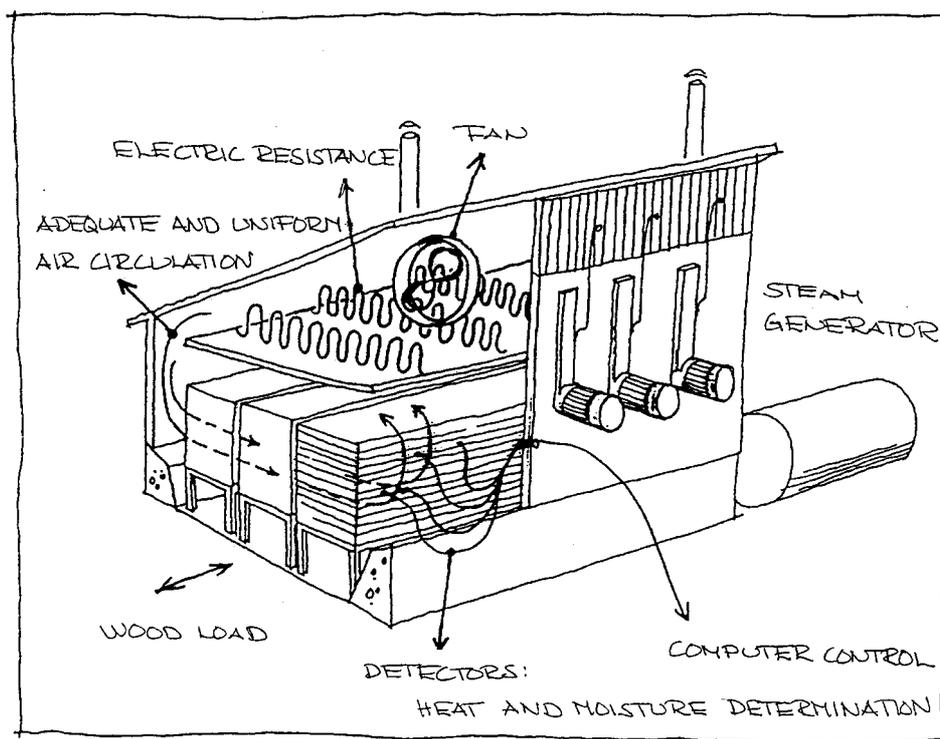
Picture 1. Principle of a heat treatment plant
